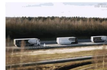
High-speed autonomous truck platooning
