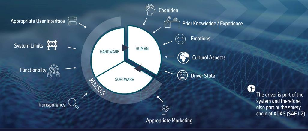
The <u>driver is part of the system</u> and needs to be <u>considered in the development of ADAS</u>. Various factors have an impact on how a human driver behaves and interacts with the system.
