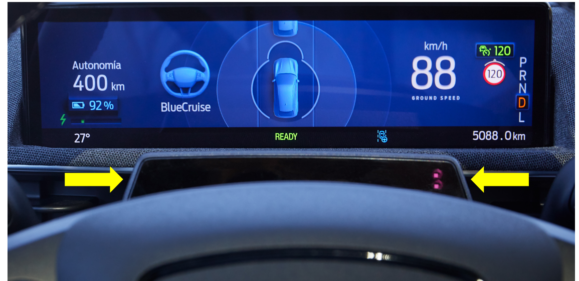
Location of Driver Facing Camera
